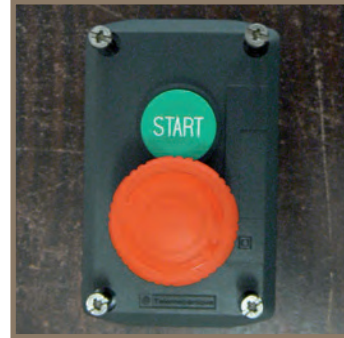
Local Start / Stop station
